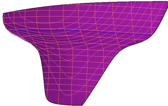
**Fig. 2** MaxiMOOP hull shape lines.
