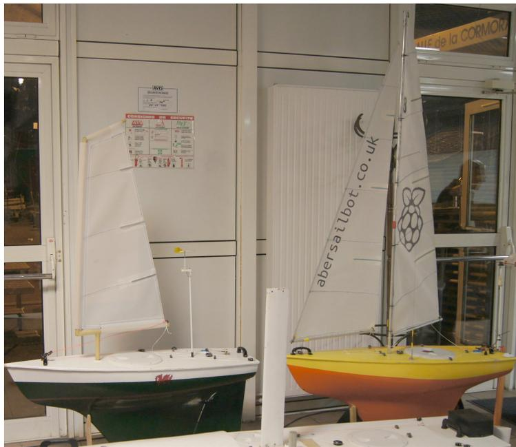
**Fig. 3** Morwyn (left) and Dewi (right) showing attached and transom-hung rudders.
