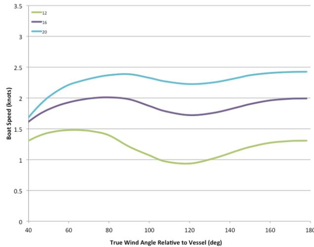
**Fig. 9** Predicted MaxiMOOP performance versus wind angle in wind speeds of 6 to 20 knots with the 0.24m<sup>2</sup> voyaging sail and higher centre of gravity and 20.5 kg displacement.
