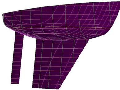
**Fig. 13** Proposed lines of an improved MaxiMOOP.
