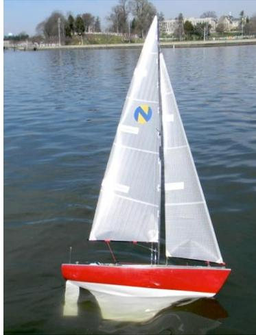
**Fig. 4** Mid Life Crisis showing spade rudder design and racing sloop rig.
