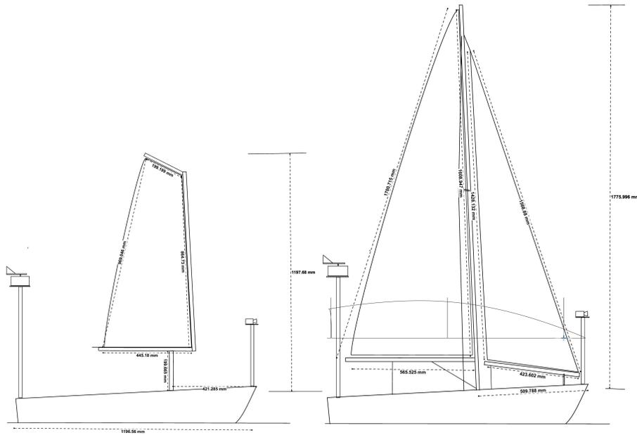
**Fig. 5** Racing sloop rig (left) and free standing, rotating balanced gaff rig (right).
