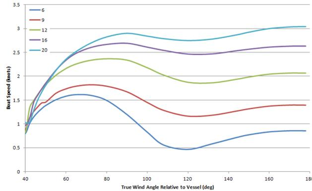
**Fig. 8** Predicted MaxiMOOP performance versus wind angle in wind speeds of 6 to 20 knots with the 1.0m<sup>2</sup> racing rig, lower centre of gravity and 16kg displacement.
