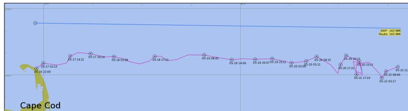
**Fig. 11** A showing ABoat Time's route during her 2014 Microtransat attempt from Cape Cod, Massachusetts to Fenit, Ireland. The blue line indicates a measurement of 165 nautical miles to the East of Cape Cod and the purple line represents the path followed by the boat. The text at each point indicates the date (MM-DD format) and time (HH:MM format, in UTC) that the position report was transmitted.
