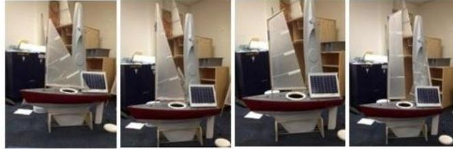
**Fig. 6** Four tested rigs: Marconi (AR=3), Marconi (AR=6), gaff (AR=3), gaff (AR=6)
