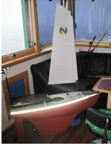
**Fig. 12** ABOat Time on board the M/V Atlantic Destiny. Her damaged solar panel is evident and the taped-over wind indicator was necessary to stop her sail and rudder from adjusting when she was hauled aboard.
